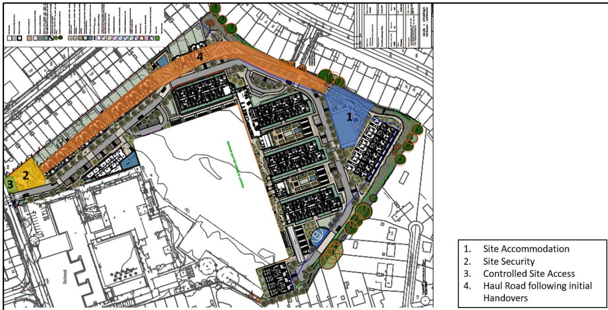
Figure 5.1 Proposed Site Compound & Staff parking Location.
